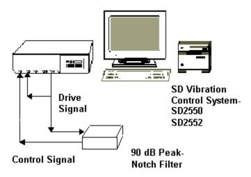
Figure 3: Closed-loop random control test setup
