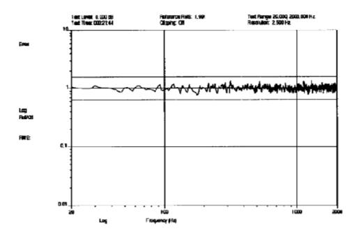
Figure 5: Error spectrum of control with <u>+</u> 2 dB tolerances
