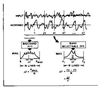
Figure 11 — Band Selectable Fourier Analysis<sup>®</sup> versus baseband Fourier analysis. BSFA processes more data to obtain increased frequency resolution.
