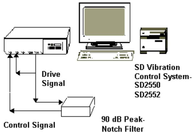
Figure 3: Closed-loop random control test setup
