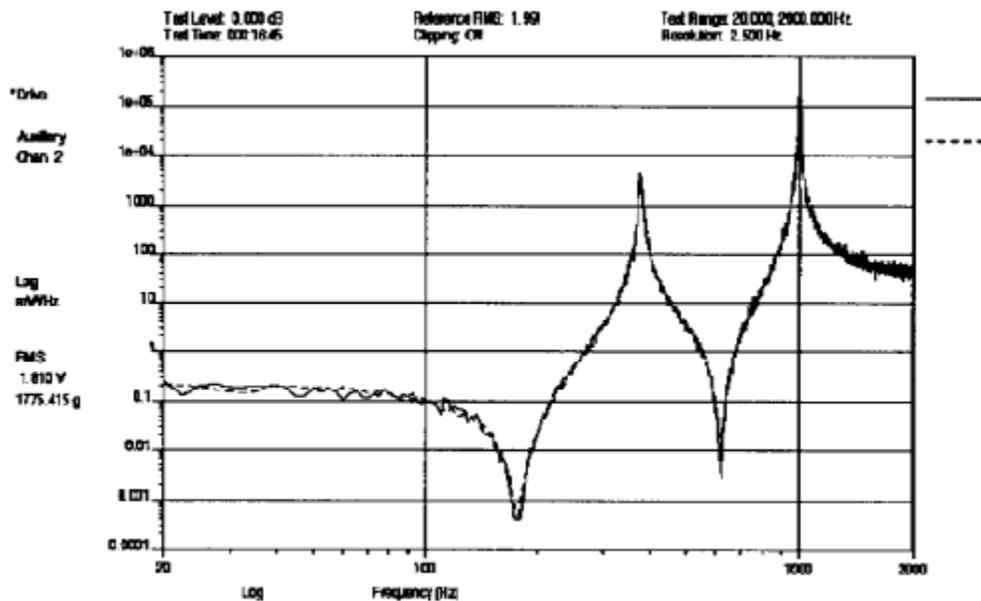
**Figure 6: Drive spectrum as reported by control system and measured as an auxiliary input channel**
