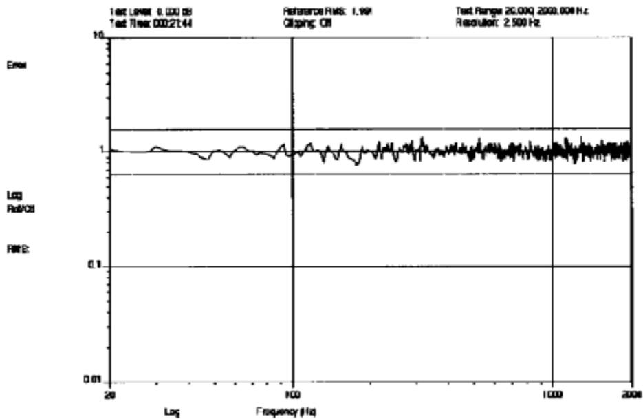
Figure 5: Error spectrum of control with  $\pm 2$  dB tolerances
