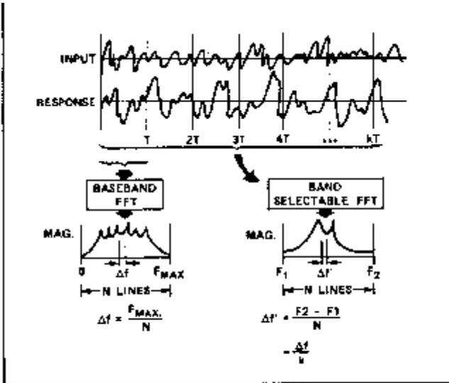
Figure 11 — Band Selectable Fourier Analysis<sup>SM</sup> versus baseband Fourier analysis. BSFA processes more data to obtain increased frequency resolution.
