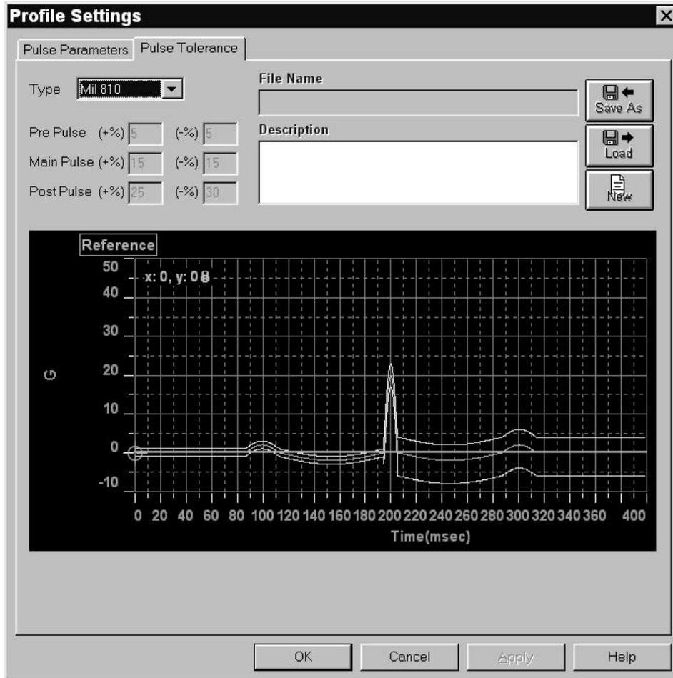
Figure 4-4. Pulse Tolerance Tab of the Profile Settings Window.
