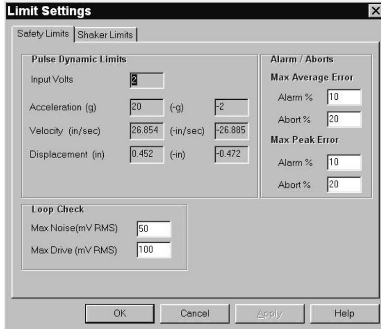
Figure 4-7. Safety Limits Tab on the Limit Settings Window
