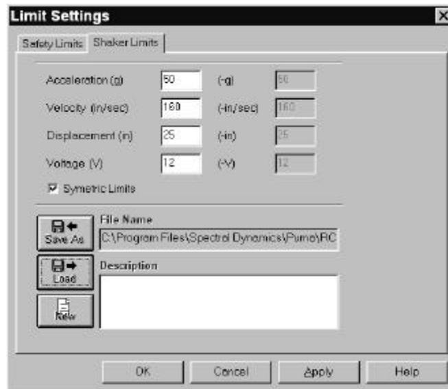
Figure 4-8. Shaker Limits Tab of the Limit Settings Window
