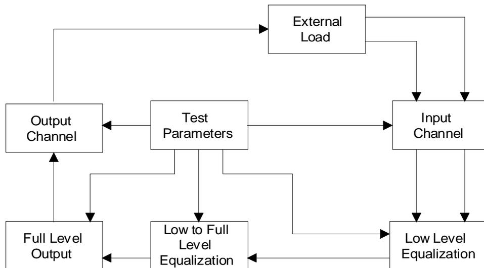
Figure 2-1. Shock Synthesis Control Loop Diagram
