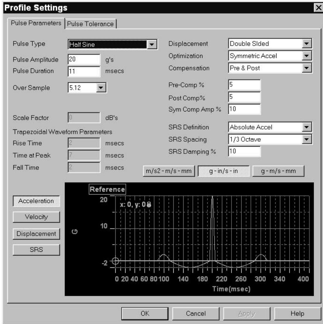
Figure 4-3. Pulse Parameters Tab of Profile Settings Window
