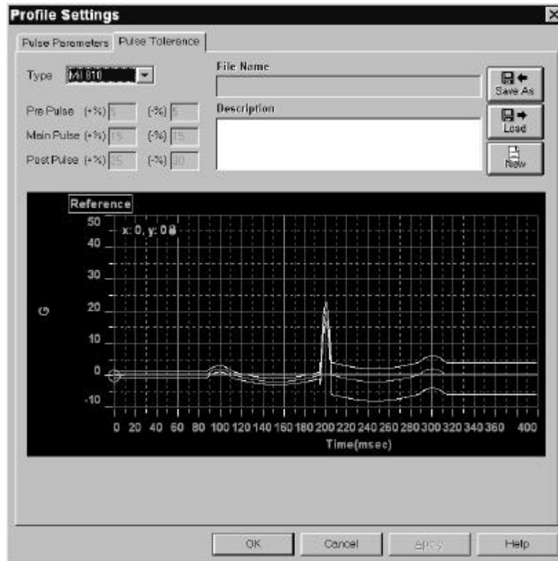
Figure 1-8. Pulse Tolerance Tab of the Profile Settings Window
